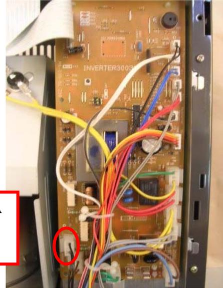
RETIRER LA CONNECTIQUE DE LA SOUFFLERIE SUR LA PLATINE ELECTRONIQUE
